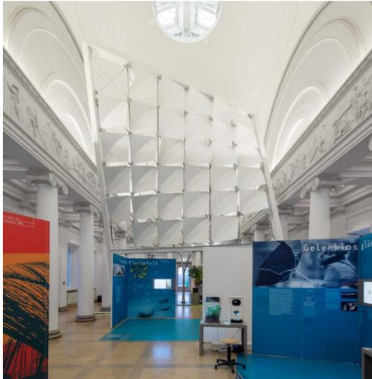
Fig. 2: Impression of the 6x6m large demonstrator of the Flectofold façade shading system inspired by the closing mechanism of the waterwheel plant and developed in the A04-project at the TRR 141 exhibition in the State Museum of Natural History in Stuttgart. © PBG & SMNS
