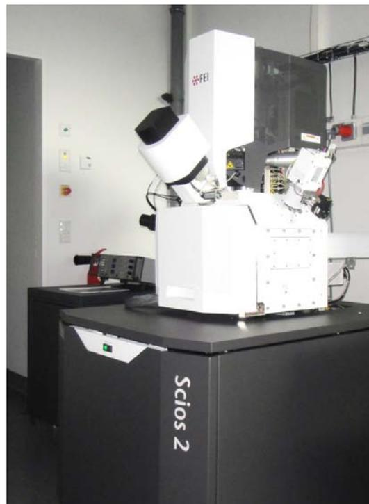
Fig. 4: FIB / SEM system Scios 2 in the FIT (© Thomann)
