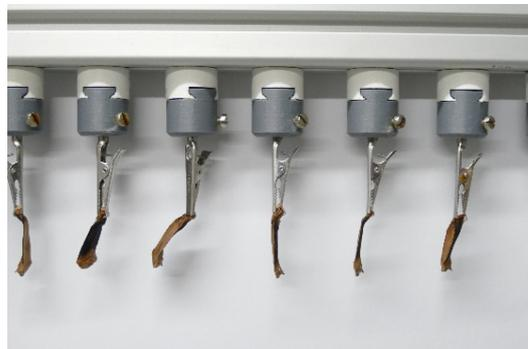
**Fig. 1:** Six cone scales of *Pinus jeffreyi* are mounted in the pine cone submerger. During our experimental timeline each scale completed 102 cycles of actuation. During each cycle they were first submerged in water for 90 min and then dried in front of a fan for 4,5 h. (© Plant Biomechanics Group)
