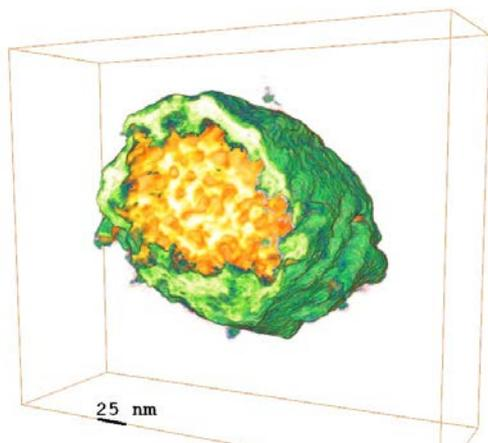
**Fig. 3:** TEM tomography of a nanoparticle with a mesoporous carbon core (orange) and a polymer shell (green). The internal structure of the particle is revealed by virtual sectioning of the particle in Avizo® software. (sample: N. Ortlieb / group Prof. A. Fischer) Image © R. Thomann
