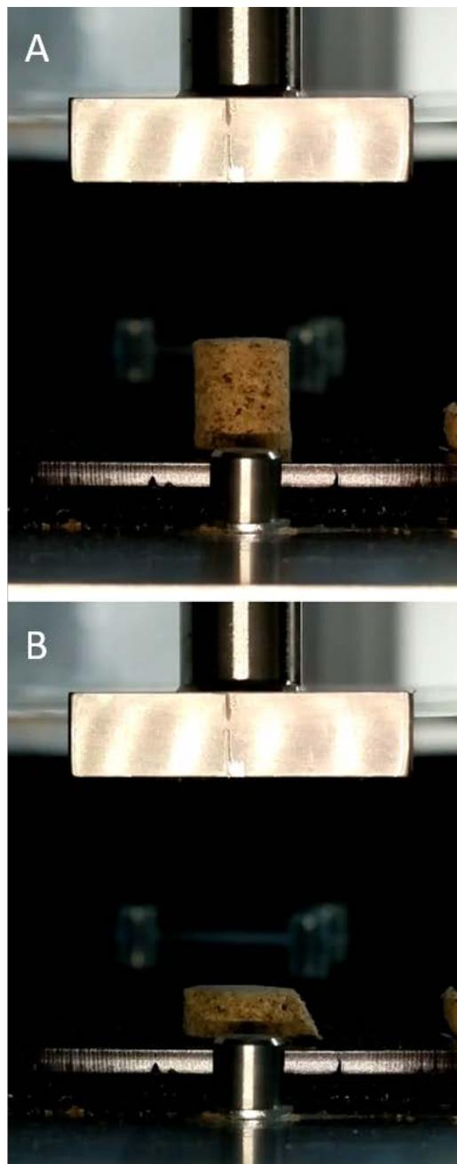
**Fig. 1:** Automated compression tests of a specimen provided by the sample wheel. (A) Intact sample. (B) Destroyed (compressed) sample. (c) Plant Biomechanics Group Freiburg
