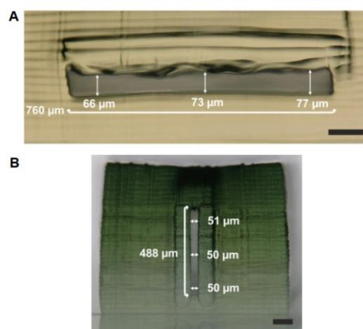
**Fig. 3:** Different aspect ratio microchannels fabricated with a custom 3D printing strategy. (A) Microchannel with an aspect ratio of 0.1, printed by in-plane manipulation of the illumination dose. (B) Microchannel with an aspect ratio of 10, printed by in-plane manipulation of the beam size. Scale bars 100  $\mu\text{m}$ . (© Neptunlab, IMTEK)
