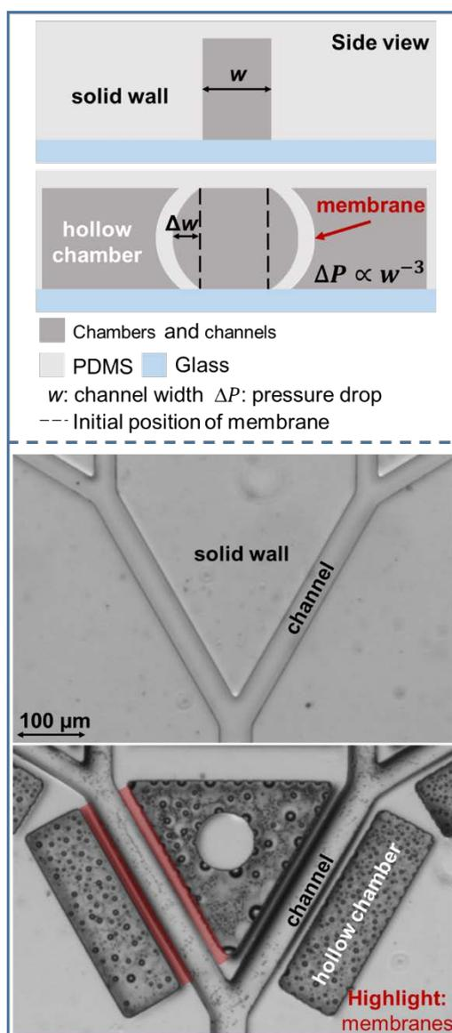
**Fig. 2:** Working principle of tuning local elasticity in a single layer (top). Resulting structures after replica molding (bottom) with water flowing through the channels. © Pfohl Group
