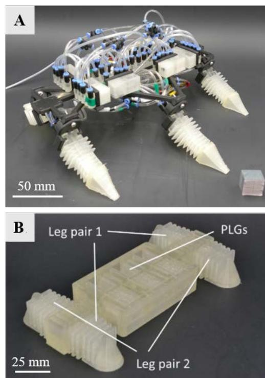
**Fig. 2:** Soft robotic walkers controlled by PLGs. A: Stick insect inspired compliant robot featuring six insect inspired leg actuators on a rigid frame controlled by 8 PLGs to achieve forward locomotion. Adapted with permission by Springer-Verlag from [4] B: Soft walker printed in one process on an FDM printer with an integrated oscillator of three PLGs [3].
