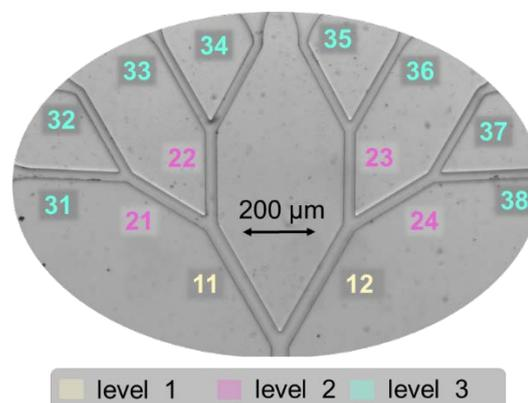
**Fig. 1:** Design of an optimized network. Widths are chosen based on the constructal law. Numerical indicators are used to identify different branches on the same construct level. © Pfohl Group
