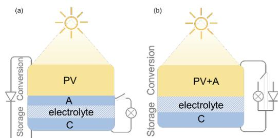
**Fig. 1:** Schematic diagram of the Mode II (a) and Mode III (b) photostorage devices. © *livMatS* / Daniel Hellweg
