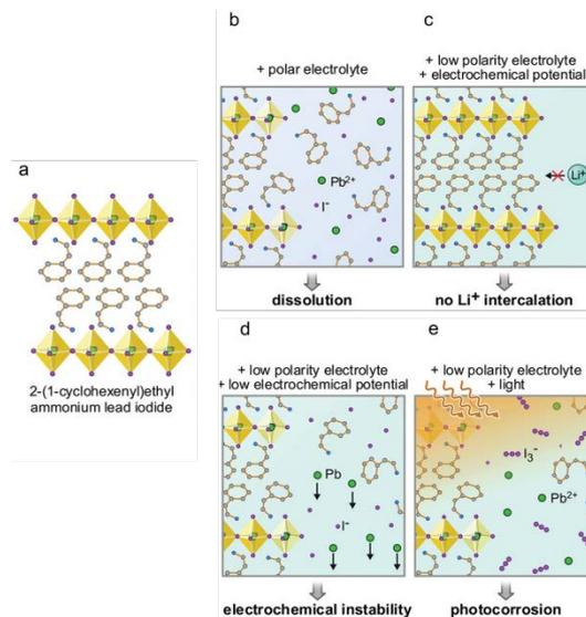
**Fig. 3:** Schematic of the demonstrated CHPI behaviour for different scenarios. (a) Simplified schematic structure. (b) Dissolution in polar solvents. (c) Stability in low polarity electrolytes, but no quantitative  $\text{Li}^+$  intercalation. (d) Reductive electrochemical degradation by  $\text{Pb}^0$  formation. (e) Photo corrosion under illumination. Adapted from [2]
