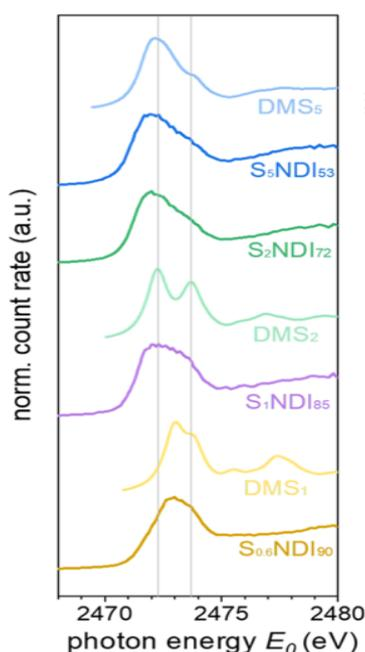
**Fig. 2:** Comparison of experimental XAS spectra of LiS cathode materials ( $S_xNDI_y$ ) and simulated spectra ( $DMS_z$ ) reveals the S-chain length  $z$  [3] (© 2023 The Authors. ACS Applied Energy Materials)
