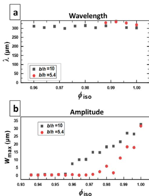
**Fig. 4:** Graphical representation of (a) wavelength variations and (b) amplitude variations with changes in the volume fraction of isopropanol. © Pfohl Group
