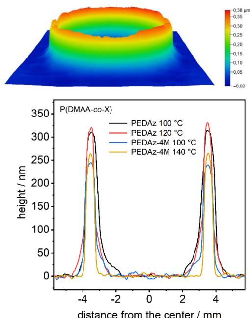
**Fig. 5:** Top: White light interferometer images (WLI) of thermally structured P(DMAA-co-PEDAz). Bottom: Height profiles of the rings obtained by thermal structuring at constant conversion. Increasing the temperature and use of the more reactive crosslinker PEDAz-4M improves the resolution. © CPI, IMTEK Univ. of Freiburg.
