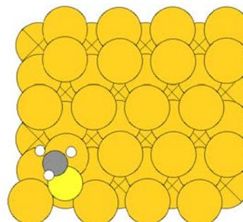
**Fig. 1:** Hollow configurations of SCH3 molecule on Gold surface (FCC111) (© Modelling and Simulation of Materials Systems Group)
