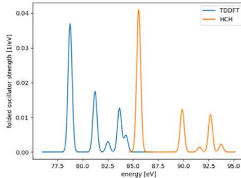
**Fig. 1:** The simulated XAS spectra of 2s transition for the Mg atom. The spectra produced by the newly implemented  $\Delta$ -KS HCH method are in orange, and the spectra produced by TDDFT in blue. (© Modelling and Simulation of Materials Systems Group)
