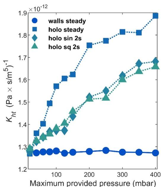
**Fig. 4:** Total hydrodynamic conductivity versus pressure calculated under a steady applied pressure profile for the solid walls device and for sinusoidal, square pulse train and steady applied pressure profiles for the holoelastic device. A maximum improvement of up to 45 % can be observed for the hydrodynamic conductivity. © Pfohl Group
