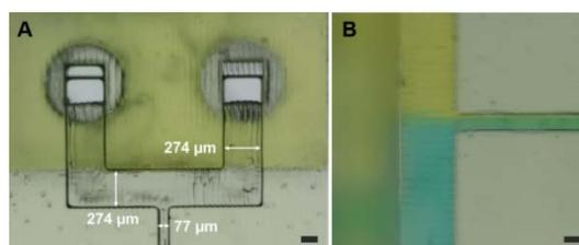
**Fig. 4:** 3D printed microfluidic mixer. (A) Microchip inlet displaying the reduced channel width of 77  $\mu\text{m}$ . (B) Microchip perfused with yellow and blue dye at a flowrate of 0.1  $\mu\text{l}/\text{min}$ . Both liquids mix readily due to the small volume. Scale bars 100  $\mu\text{m}$ . (© Neptunlab, IMTEK)
