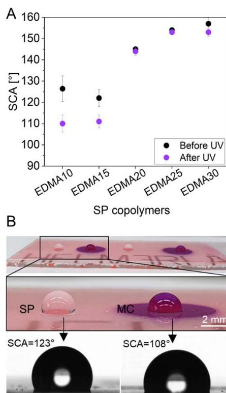
**Fig. 2:** Photoswitchable wetting properties of our SP copolymers. A) SCA values of SP copolymers with different EDMA content, i.e. different pore size and roughness. B) A circular area on the sample EDMA10 was switched to MC by UV light and the SCA of two  $5\ \mu\text{l}$  water droplets was compared. (© HelmerLAB, IMTEK)
