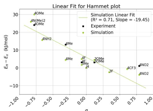
**Fig. 3:** The calculations of the activation energy of carbenes with various substituents, show that the difference  $E_H - E_X$  is linear in the Hammett parameter  $\sigma$ , where  $\sigma > 0$  corresponds to electron-withdrawing effects of the substituent, while  $\sigma < 0$  indicates electron-donating effects. This linear relation can be used to predict the activation energy  $E_X$  of carbenes with any substituent X. (© Modelling and Simulation of Materials Systems Group)
