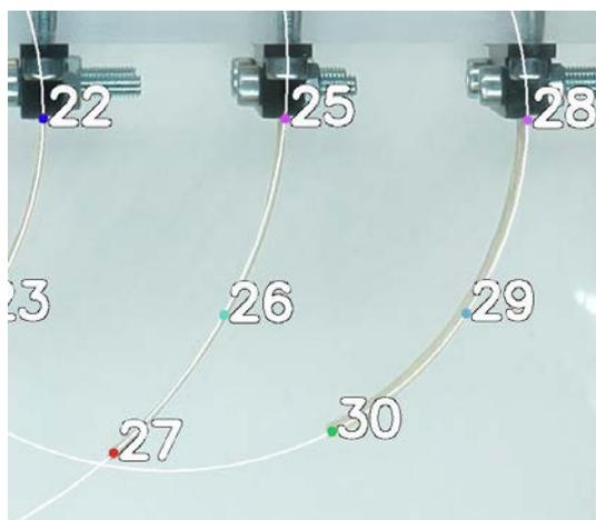
**Fig. 2:** Ten 3D-printed hygroscopic actuators were mounted in a climate chamber for an experimental series of five temperature steps ranging from 10 to 50°C. For each temperature step, the relative humidity was systematically increased from 15% to 95%. During this series of experiments, the curvature of the demonstrators was calculated using a custom-made tracking tool and three markers (numbered points, e.g. 25-27) on the outer edge of each specimen. (© Plant Biomechanics Group)
