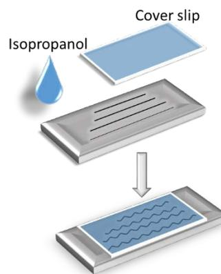
**Fig. 2:** Schematic representation of the step-by-step experimental procedure, illustrating the systematic process from the placement of the microfluidic device to the observation of the membrane response under varying isopropanol/water volume fractions. © Pfohl Group
