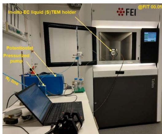
**Fig. 1:** In-situ Electrochemical Liquid (Scanning) Transmission Electron Microscopy set-up installed and run by the Fischer group at the core facility "Imaging of material systems" at FIT. Image copyright ©AK Fischer. All rights reserved.
