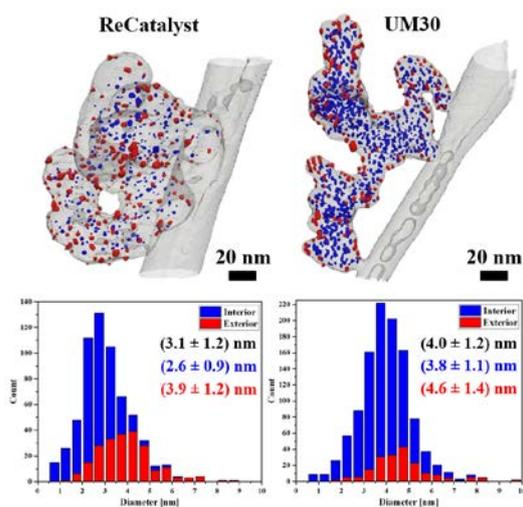
**Fig. 1:** Segmented volumes of a ReCatalyst (left) and a UM30 PtCo/C particle (right) and corresponding particle size distributions with subdivision of nanoparticles into interior (blue) and exterior (red). (© Electrochemical Energy Systems Group)
