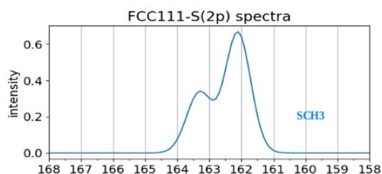
**Fig. 2:** XPS Analysis of S(2p) Spectra for bound  $\text{SCH}_3$  Thiol on the FCC111 Gold surface (Simulation), compare to the XPS S(2p) Spectra for C16 bound Thiol in experiment, Fig. 1 in Ref. [5]. (© Modelling and Simulation of Materials Systems Group)
