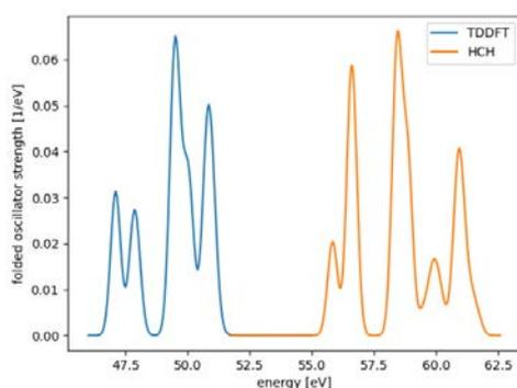
**Fig. 2:** The simulated XAS spectra of  $2p$  transition for the Mg atom. The spectra produced by the newly implemented  $\Delta$ -KS HCH method are in orange, and the spectra produced by TDDFT in blue. (© Modelling and Simulation of Materials Systems Group)
