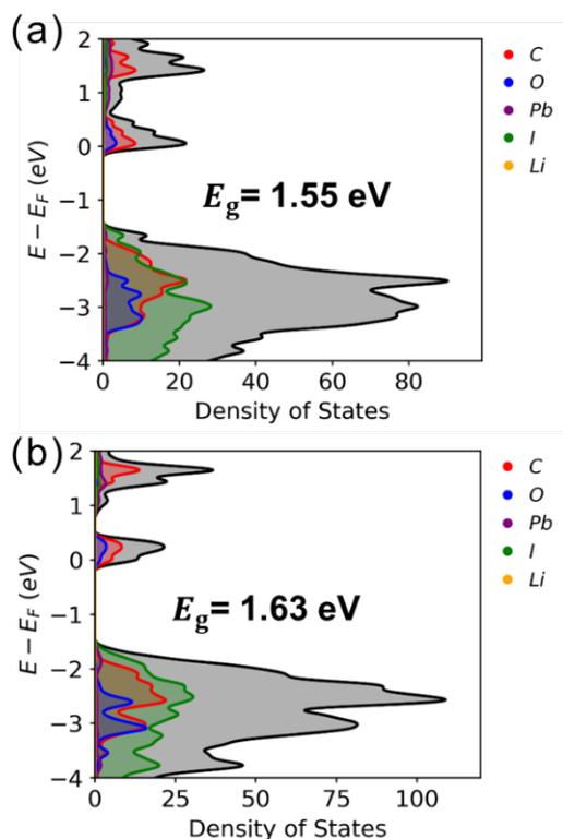
**Fig. 3:** Electronic DOS for the (1/2, 1/2) displaced model with a Li atom inserted (a) into the inorganic octahedral void; (b) close to the oxygen atom of the inorganic DA spacer. The color code follows Figure 2. There is no substantial Li contribution (orange) visible in the plotted energy range. © C. Elsässer's Group
