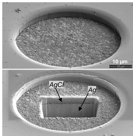
**Fig. 2:** FIB/SEM cross-sectional imaging of a micropatterned Ag/AgCl microelectrode-cavity-array, a sensor which is used in a mini electronic device for electrophysiological measurements. (sample: T. Ensslen / group Prof. Behrends, Membrane Physiology, University Freiburg). Image © Y. Thomann
