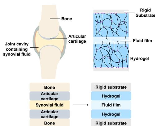
**Fig. 7:** Analogy of the natural system, the synovial joint, with the technical system, surface-attached hydrogels in Gemini contact. © CPI, IMTEK Univ. of Freiburg.
