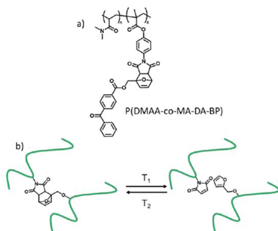
**Fig. 3:** a) Molecular structure of P(DMMA-co-MA-DA-BP); b) Reversible crosslinking behavior of MA-DA-BP. (© CPI, IMTEK Univ. of Freiburg.)
