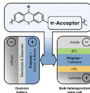
**Fig. 2:** Bifunctional phenothiazine donor-acceptor conjugated co-polymers with PV or battery functionality. Reproduced from [1]
