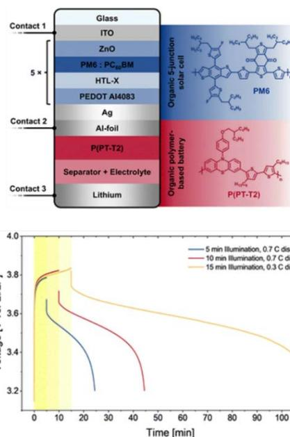
**Fig. 4:** Schematic layer sequence in the organic photobattery (top) and photocharge and discharge profiles with different illumination times and different discharge rates. Adapted from [6].
