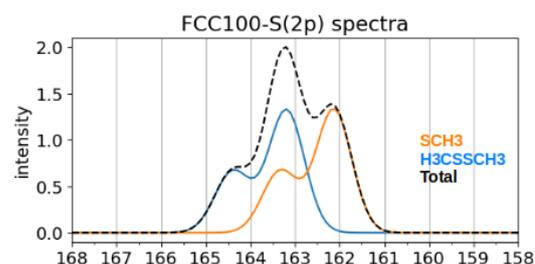
**Fig. 3:** XPS Analysis of S(2p) Spectra for bound  $\text{SCH}_3$  and unbound  $\text{H}_3\text{CSSCH}_3$  Molecules on the FCC100 Gold surface (Simulation), compare to the XPS S(2p) spectra for PMMPS bound and unbound Thiol in experiment, Fig. 1 in Ref. [5]. (© Modelling and Simulation of Materials Systems Group)
