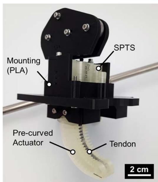
**Fig. 10:** The pneumatic actuator system with avian-inspired tendon locking mechanism (TLM). (© Plant Biomechanics Group)
