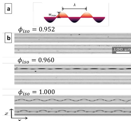
**Fig. 3:** (a) Schematic representation of the membrane buckling dynamics with amplitude as  $w_{max}$  and wavelength as  $\lambda$ , (b) microscopic images capturing the dynamic response of the membrane at different volume fractions of isopropanol, revealing distinct morphological changes in the buckling behavior. © Pfohl Group
