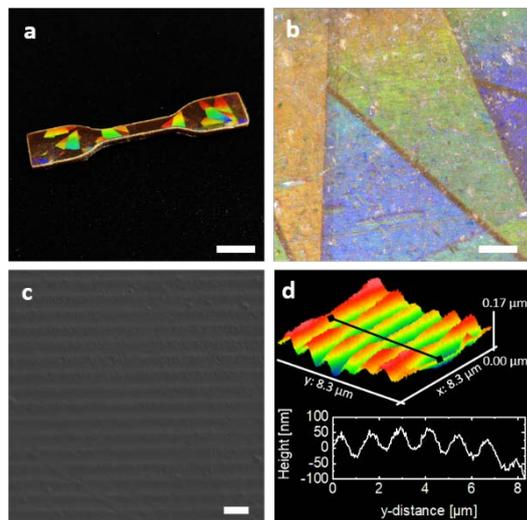
**Fig. 2:** Analysis of submicron-structured surface of COLOR3D printed wood composite by optical camera (a) optical microscopy (b), SEM (c) and WLI with the corresponding height profile (d) Scale bars: (a) 1 cm, (b) 200  $\mu\text{m}$ , (c) 2  $\mu\text{m}$ . (© Laboratory of Process Technology).
