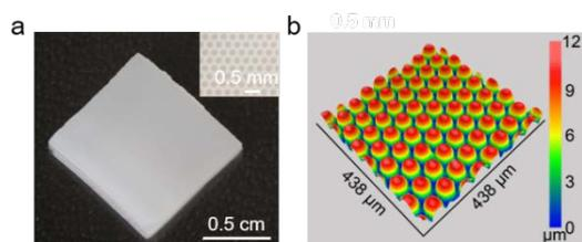
**Fig. 2:** Microstructured surface characterization. (a) The optical picture of DNH and the microscope image (inset); (b) 3D structure of the microstructure obtained via WLI. (© Neptunlab, IMTEK)
