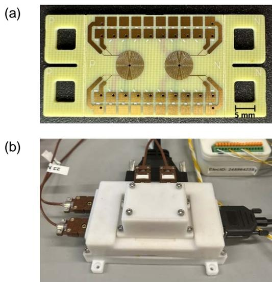
**Fig. 1:** (a) Top view of the ZT-Card PCB (b) Overview of the setup for the measurement platform which consists of thermocouples, thermocouple holders, spring contacts, DSub connectors and the ZT-Card. © IMTEK/Laboratory for Design of Microsystems
