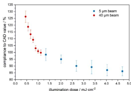
**Fig. 1:** Accordance of 3D printed calibration structure dimensions to the CAD dimensions. Both the high-resolution 5  $\mu\text{m}$  beam and the lower resolution 40  $\mu\text{m}$  beam show the closest accordance around 1.2  $\text{mJ}\cdot\text{cm}^{-2}$ . © Neptunlab, IMTEK
