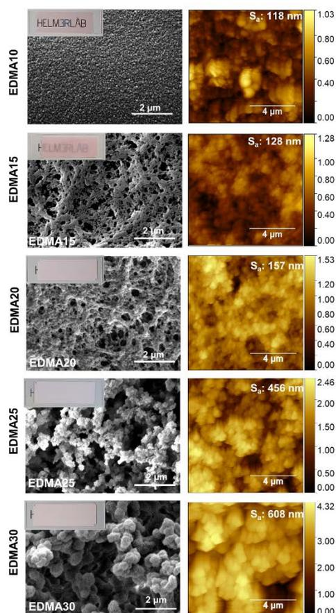
**Fig. 1:** Surface characterization of SP copolymers with different pore sizes. A) SEM images and B) AFM measurements (lateral scale in  $\mu\text{m}$ ) of SP copolymers. Increasing EDMA content resulted in larger pore size, i.e. larger roughness parameters ( $S_a$ ). Insets: Photograph of the SP copolymer thin films. (© HelmerLAB, IMTEK)
