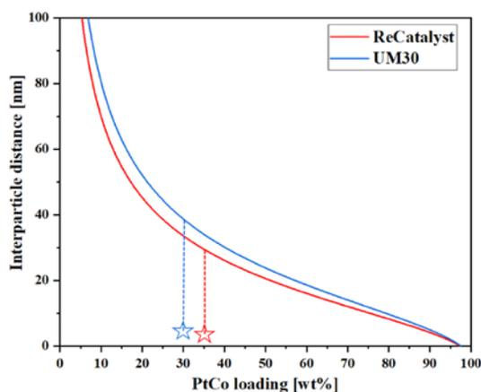
**Fig. 3:** Calculation of border-to-border interparticle distances via the approach of Meier *et al.*<sup>6</sup> for PtCo nanoparticles using the determined average nanoparticle sizes and assuming densities of  $\rho_{\text{Pt}} = 21.45 \text{ g/cm}^3$  and  $\rho_{\text{Co}} = 8.90 \text{ g/cm}^3$  and a surface area of  $800 \text{ m}^2\text{g}^{-1}$  for the carbon support. The hollow stars depict the obtained distances by STEM 3D analysis. (© Electrochemical Energy Systems Group)
