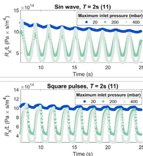
**Fig. 3:** Temporal evolution of hydrodynamic resistance in branch 11 of a holoelastic device under a sinusoidal (top) and square pulse train (bottom). Minimum values are achieved for the highest applied pressure. © Pfohl Group
