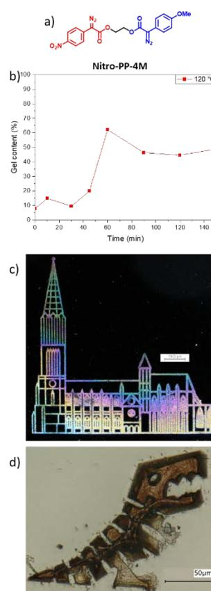
**Fig. 2:** a) Molecular structure of **Nitro-PP-4M**; b) Crosslinking of a modified PDMAA with **Nitro-PP-4M** at 120 °C; c) Photolithography of a modified PU with **Nitro-PP-4M**; d) Printed dinosaur made with 2 photon lithography from modified lignin. (© CPI, IMTEK Univ. of Freiburg.)
