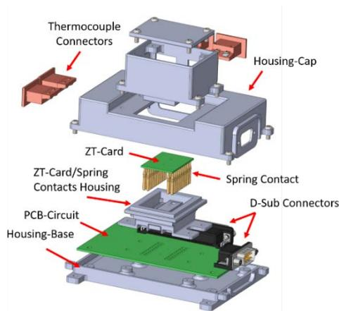
**Fig. 2:** Exploded view of the measurement housing platform. © IMTEK/Laboratory for Design of Microsystems
