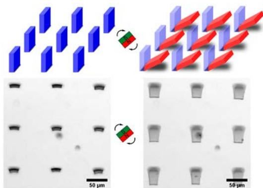
**Fig. 2:** Schematic illustration and light microscopy images of beam-like magnetic microactuators written with 2PC and actuated under a rotating external magnetic field. © CPI, IMTEK Univ. of Freiburg.
