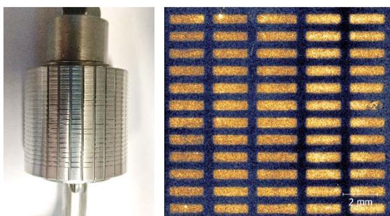
**Fig. 6:** Structured aluminum roll and a fluorescence microscopy image of a substrate patterned by a roll-to-roll process. © CPI, IMTEK Univ. of Freiburg.
