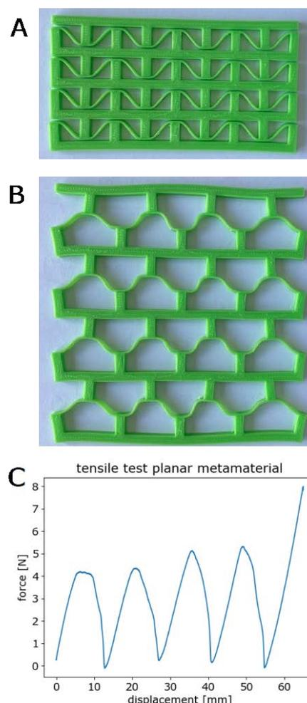
**Fig. 1:** A. Planar topology flexible mechanical metamaterials at resting state, B. fully snapped stable state. C. Tensile test curve of the metamaterial depicted in subfigures A and B, snap-through instability occurs for each line of unit cells. (© Laboratory for Soft Machines)
