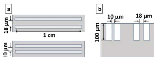
**Fig. 1:** Illustration depicting the configuration of the PDMS microfluidic device. (a) Top view displaying two vertically oriented membranes of 10  $\mu\text{m}$  and 18  $\mu\text{m}$  thickness  $h$ , each 1 cm long. (b) Side view with the membrane height  $b$  set to 100  $\mu\text{m}$ . © Pfohl Group
