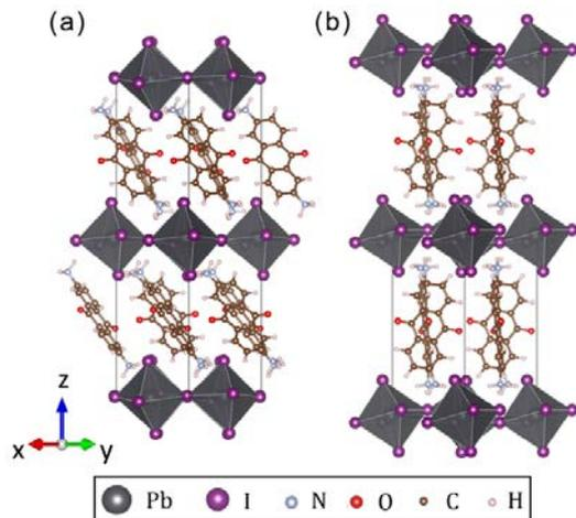
**Fig. 1:** The atomistic models for the DJ phase in 2,6-diammonium anthraquinone lead iodide (DAPbI) with (a) the ( $1/2, 1/2$ ) displaced stacking of the inorganic layers and (b) the (0, 0) displaced stacking of the inorganic layers.. © C. Elsässer's Group
