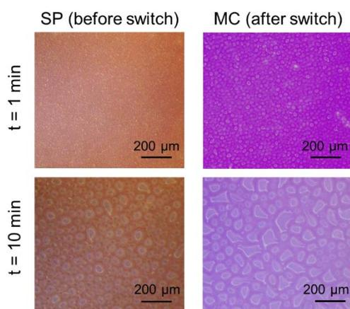
**Fig. 3:** Water vapor condensation on EDMA10 before and after UV, 1 min and 10 min after exposure to humidity. Larger number of droplets form and coalesce on MC surface. (© HelmerLAB, IMTEK)
