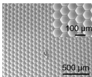
**Fig. 3:** Optical application illustration of the microfabrication method. SEM images of the replicated PDMS microlens array under different magnifications. (© Neptunlab, IMTEK)
