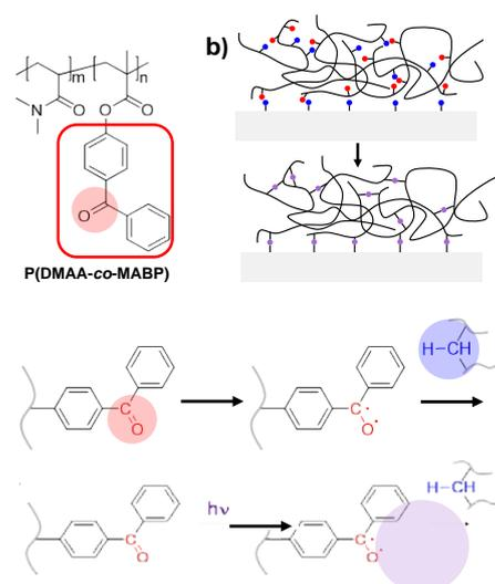
**Fig. 8:** a) Molecular structure of poly(dimethylacrylamide-co-methacryloxybenzophenone). b) Surface-attachment and hydrogel formation via CHic. c) Reaction mechanism of C-H insertion crosslinking (CHic). © CPI, IMTEK Univ. of Freiburg.
