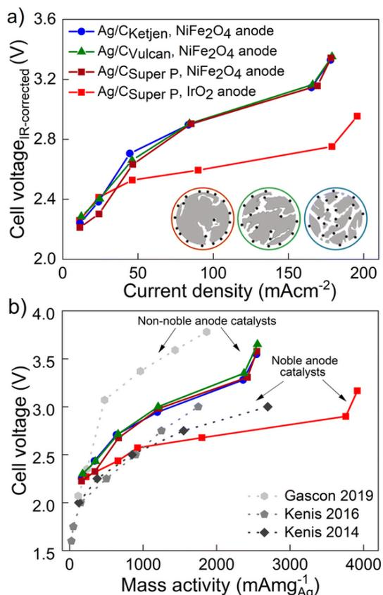
**Fig. 2:** (a)  $iR$ -Corrected cell voltage over CO partial current density for Ag/C<sub>Ketjen</sub>, Ag/C<sub>Vulcan</sub> and Ag/C<sub>Super P</sub> catalysts in 0.1 M KOH at ambient temperature. (b) CO partial current density relative to Ag loading of selected supported Ag catalysts achieving high mass activities. (adapted from Seteiz *et al.* [4] CC BY Copyright © 2023)
