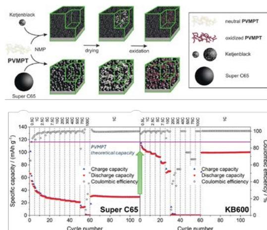
**Fig. 5:** Schematic diagram of PVMPT-carbon electrodes with Ketjenblack and Super C65 as carbon additive and resulting battery performance. Utilization of Ketjenblack instead of Super C65 results in a massive improvement in terms of the accessible specific capacity. Reproduced from [7]
