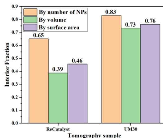
**Fig. 2:** Interior fraction of nanoparticles regarding their number, their volume and their surface area for the two examined PtCo/C species. (© Electrochemical Energy Systems Group)
