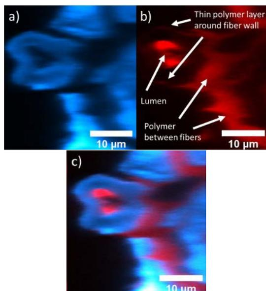
**Fig. 2:** a) CLSM picture of calcofluor white labeled paper fibers. b) CLSM picture of spatial distribution of rhodamine B labeled wet strength agent c) Z-stacking of previous CLSM pictures for a better understanding of spatial distribution of wet strength agent inside the paper. © CPI, IMTEK Univ. of Freiburg
