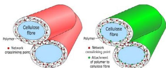
**Fig. 1:** Schematic depiction of wet strength mechanism: protection mechanism (left side in red) and reinforcement mechanism (right side in green) © CPI, IMTEK Univ. of Freiburg
