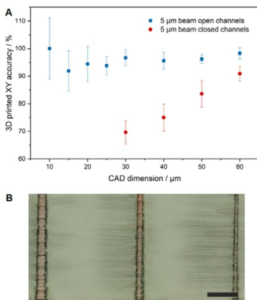
**Fig. 2:** 3D printed microchannels and achieved XY accuracy of the high-resolution 5  $\mu\text{m}$  beam. (A) Channel width of open and embedded channels compared to the corresponding CAD dimensions. Embedded channels can be printed down to a CAD dimension of 30  $\mu\text{m}$ , resulting in a 3D printed channel width of 21  $\mu\text{m}$ . (B) 3D printed microchannels down to 21  $\mu\text{m}$  filled with red dye. Scale bar 100  $\mu\text{m}$ . (© Neptunlab, IMTEK)
