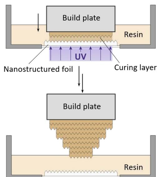
**Fig. 1:** Schematic illustration of COLOR3D printing process by DLP 3D printing of the individual layers in combination with replication of the submicron-structured foil at the bottom of each layer (© Laboratory of Process Technology).
