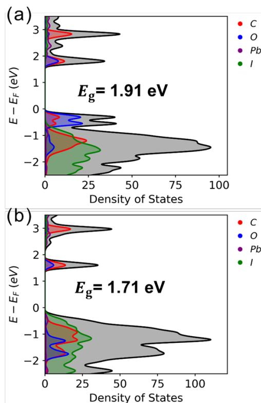
**Fig. 2:** Electronic DOS for the ( $1/2, 1/2$ ) displaced model in DAPbI (a) without and (b) with a DFT+ $1/2$  treatment of O ( $r_{\text{cut}}^{\text{O}} = 2.8$  bohr). The total DOS is shown in grey while the projected DOS of C, O, Pb, and I are shown in red, blue, indigo, and green, respectively. © C. Elsässer's Group
