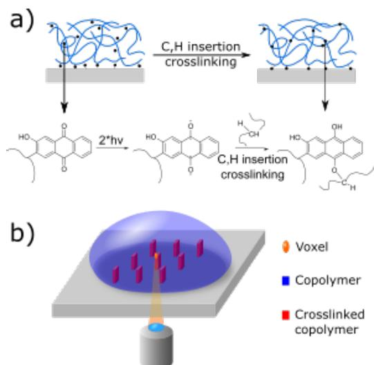
**Fig. 1:** Schematic representation of a) the C,H-insertion reaction of a reactive group (anthraquinone derivate) via a bi-radical transition state and b) the direct writing into a polymer layer by Two photon crosslinking (2PC). © CPI, IMTEK Univ. of Freiburg.
