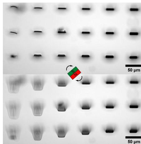
**Fig. 3:** Light microscopy images of beam-like microactuators of different thicknesses from left to right (1-6 μm), which are moving in a rotating external magnetic field. © CPI, IMTEK Univ. of Freiburg.
