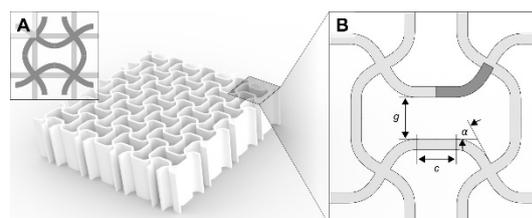
**Fig. 1:** Metamaterial and design of the unit cell. © created by D. Schwarz, published by Elsevier, unchanged from [5] under CC-BY-4.0 (<https://creativecommons.org/licenses/by/4.0/>)
