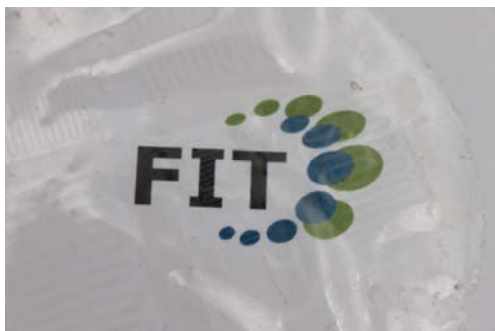
Fig. 2: Photograph of the FIT logo through a silicon foil with a structured nanowire network. © IMTEK/Laboratory for Design of Microsystems
