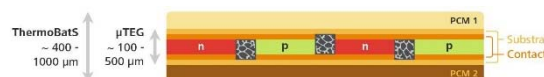
Fig. 1: ThermoBatS \mu TEG-PCM stack consisting of PCM reservoirs on top (light beige) and bottom (brown), thermally conductive substrate material (beige), contact pads (orange), TE material (red and green) and a thermally insulating polymer foam (gray). © IMTEK/Laboratory for Design of Microsystems
