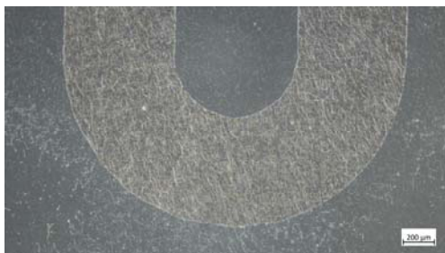
Fig. 3: Micrograph of a structured silver nanowire sheet. © IMTEK/Laboratory for Design of Microsystems
