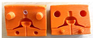
Fig. 3: The mold prototyped for molding the suction cups (© Laboratory for the Design of Microsystems, IMTEK)
