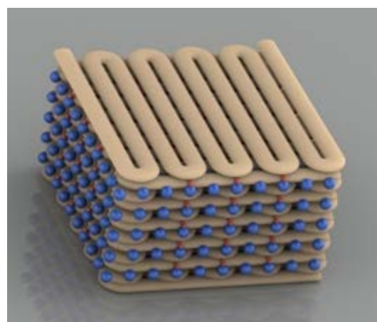
Fig. 1: Template for a hybrid bioprinting process featuring extruded ASCs (beige) and DoD-printed HUVECs (red) and thrombin (blue) for a vascularized bone tissue model characterized in vitro and in vivo . (© Cell Printing Group)
