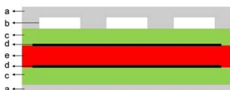
Fig. 6: Schematic of the cross-section of the bending actuator. (a) the passivation layer (b) PMMA backbones (c) elastomer layer (d) electrode layer (e) active elastomer layer for actuation (© Laboratory for Design of Microsystems)
